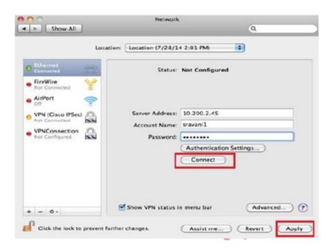
o) Enter the password configured in the gateway (under VPN Users) in the Password field and click OK
