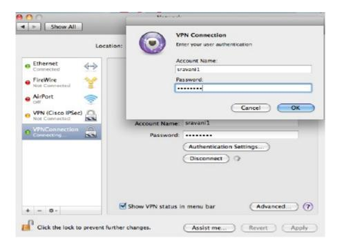
p) The VPN connection starts, and Connected displays when the connection is successful. Successful connection is indicated with green icon as shown in the following screen shot.
