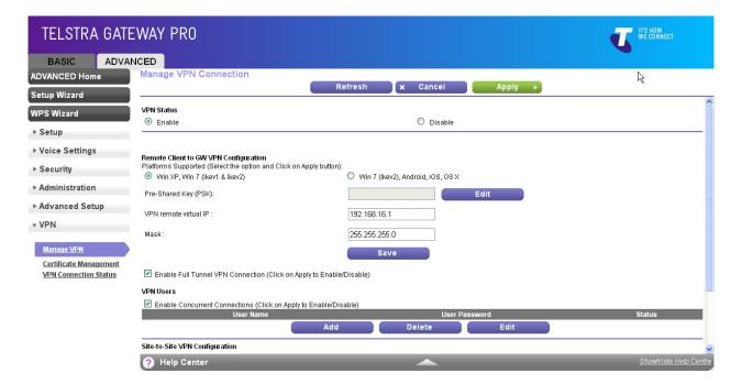
At this point, the remote client to GW VPN server feature is configured and running on the device.
