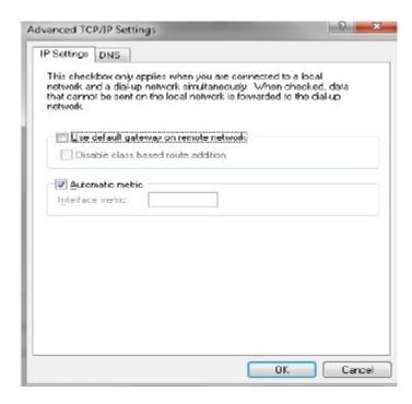
b) Split tunneling is enabled for the VPN on your Windows 7 host. If the VPN remote virtual pool configured in the V7610 GW (as shown in the following screen shot) is same as the LAN IP pool of the GW, then the VPN configuration for the split tunnel is complete. Otherwise, go to Step c.
