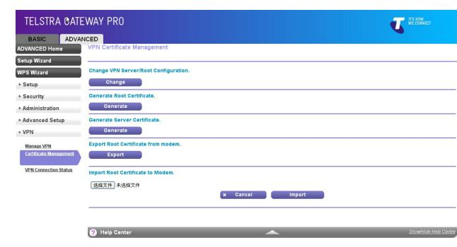
If you reset the V7610 gateway to factory defaults, the certificates generated are lost. It is possible to import the root certificate from a client computer back into the V7610. You can use the Import button on this page to restore the VPN root certificate.
