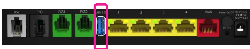
Figure 38: USB Port for Mobile Broadband Backup on side or back of device
