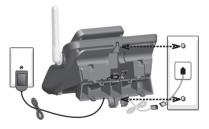
5. Slide the telephone base down until it locks securely. Bundle the telephone line cord and power adaptor cord neatly with twist ties.
