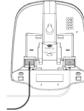
2. Check the arrow direction of the marking "Wall mount" on each of the base and the stand. Following the indicated clicking sequence, click the stand into the locking grooves at the back of the base along the arrow direction of the marking "Wall mount" until it clicks into place.
