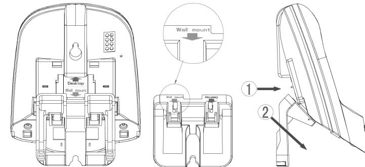
3. Thread the line cord and the power cable through the narrow space between the stand and the base to the place where they meet at the marking "Wall mount" on the base. Plug the other end of the line cord and the power cable into the telephone wall socket and the mains power socket respectively.
