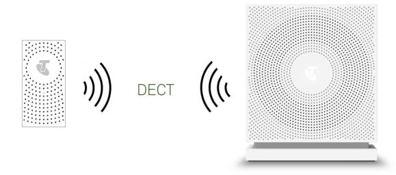
The Telstra Voice Extender (TVE) connects wirelessly via DECT to the DECT base inside your Telstra modem. The RJ11 telephone port located at the base of the TVE then provides a standard telephone wall socket in your house allowing you to connect any standard cordless or corded telephone wirelessly between the TVE and modem.
