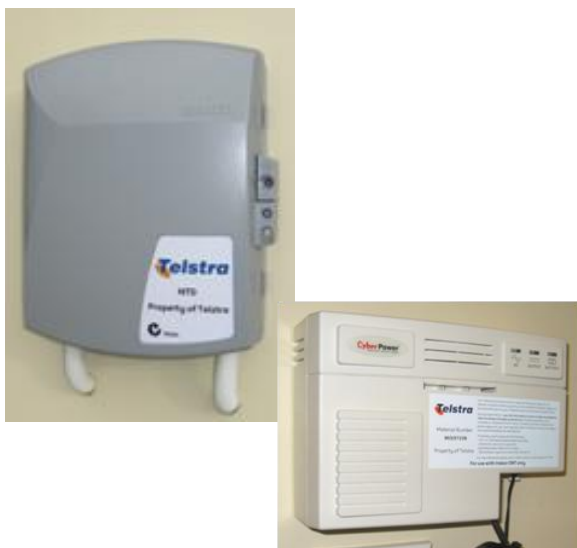
Outdoor Termination Device & Power Supply
