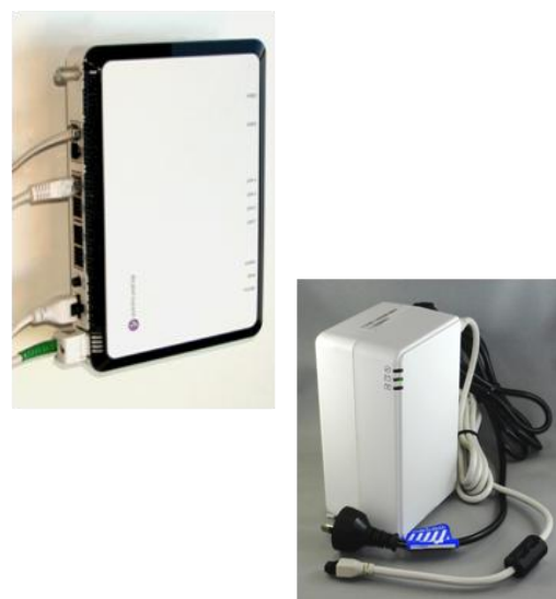
Indoor Termination Device & Power Supply
