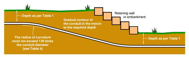
NOTE: The trenching should follow the contour of the finished ground level within the curvature (flexing) constraints of the conduit to be installed (see Table 4).
