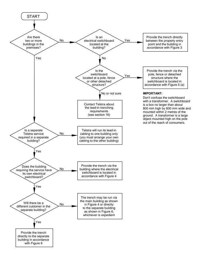
Figure 7 — Determining the appropriate method of cabling/trenching to a particular building
