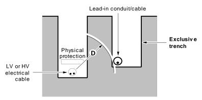
NOTE: The trench must be located such that distance "D" (refer to Table 2) is maintained between the electrical conduit or cable and the Telstra conduit/cable. This distance may be measured radially in any direction from the electrical conduit/cable.
