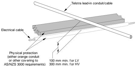
Figure 15 — Crossing ABOVE electrical cable with a protective covering that complies with AS/NZS 3000 requirements
