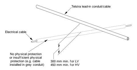
NOTE: Installation of underground electrical cable in customer premises without a protective covering is not allowable under the electrical wiring rules (AS/NZS 3000). However, there may be cases where unprotected underground electrical cable is installed.
