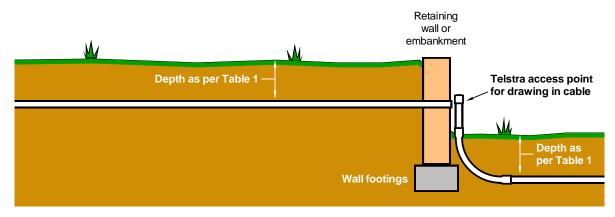
NOTE: Telstra will install conduit on the surface of the retaining wall or embankment as shown. Telstra may also install a metal cover strip over the conduit as a mower guard.
