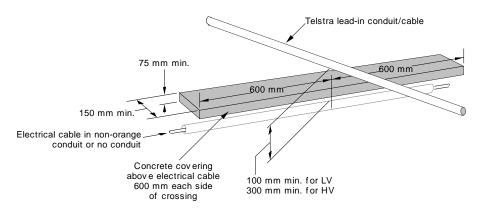
NOTE: The concrete covering is to protect against accidental contact with the electrical cable if excavating along the path of the Telstra lead-in cabling subsequent to its initial installation.
