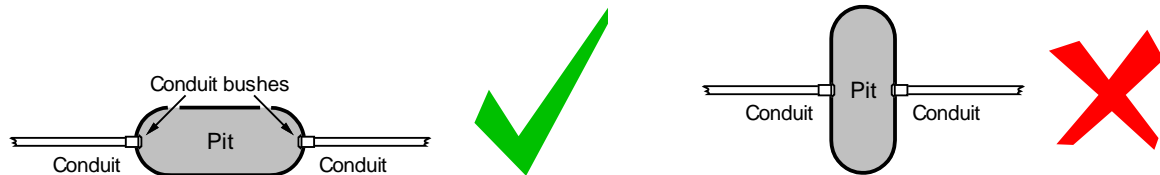
Figure 5 Right and wrong use of intermediate pits
