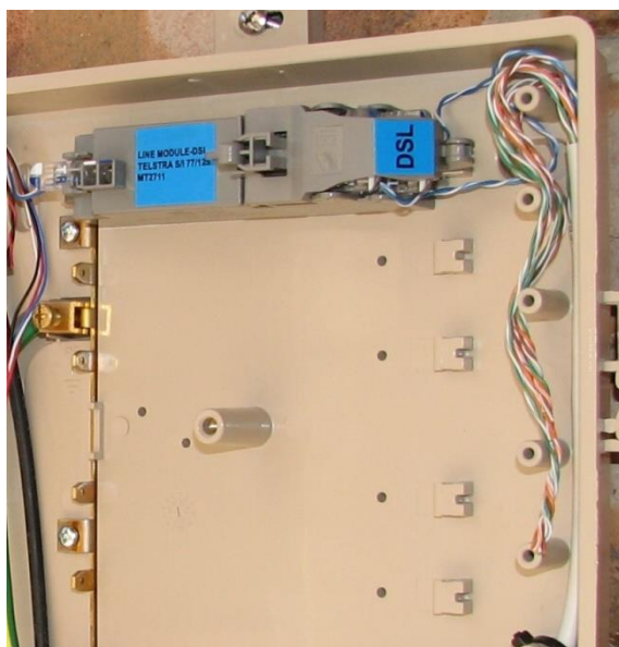
Figure 6 Central filter installed within a Telstra NTD (a) DSL line module (b) Filter in the customer compartment
