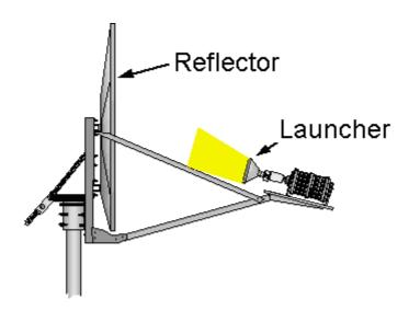
EME Clearance Zone – 35cm from the launcher towards the reflector
