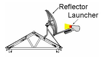
EME Clearance Zone 30cm from the launcher towards the reflector
