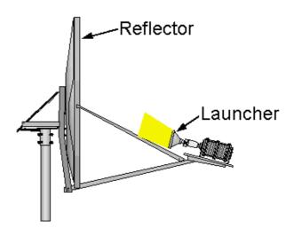
EME Clearance Zone – 40cm from the launcher towards the reflector
