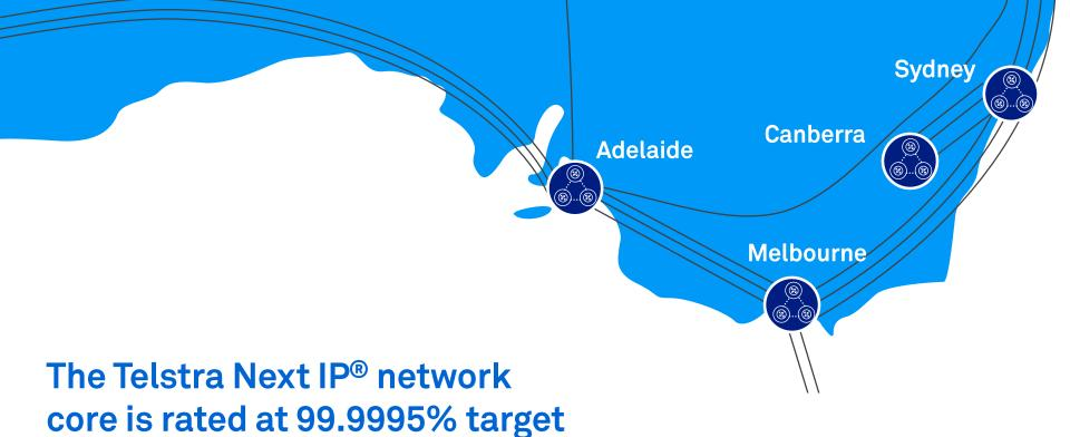
A triple-path ladder topology, with three inter-connected Provider (P)-routers at each major location. The triple path topology protects against simultaneous dual-path failure.
