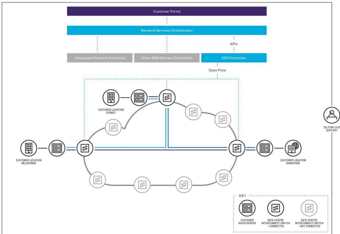
DCI uses Network Services Orchestrator and an Open Daylight-based SDN Controller using Open Flow as a control plane and Layer-2 Ethernet as the forwarding plane. The simplified diagram showing end-to-end architecture is shown below:
