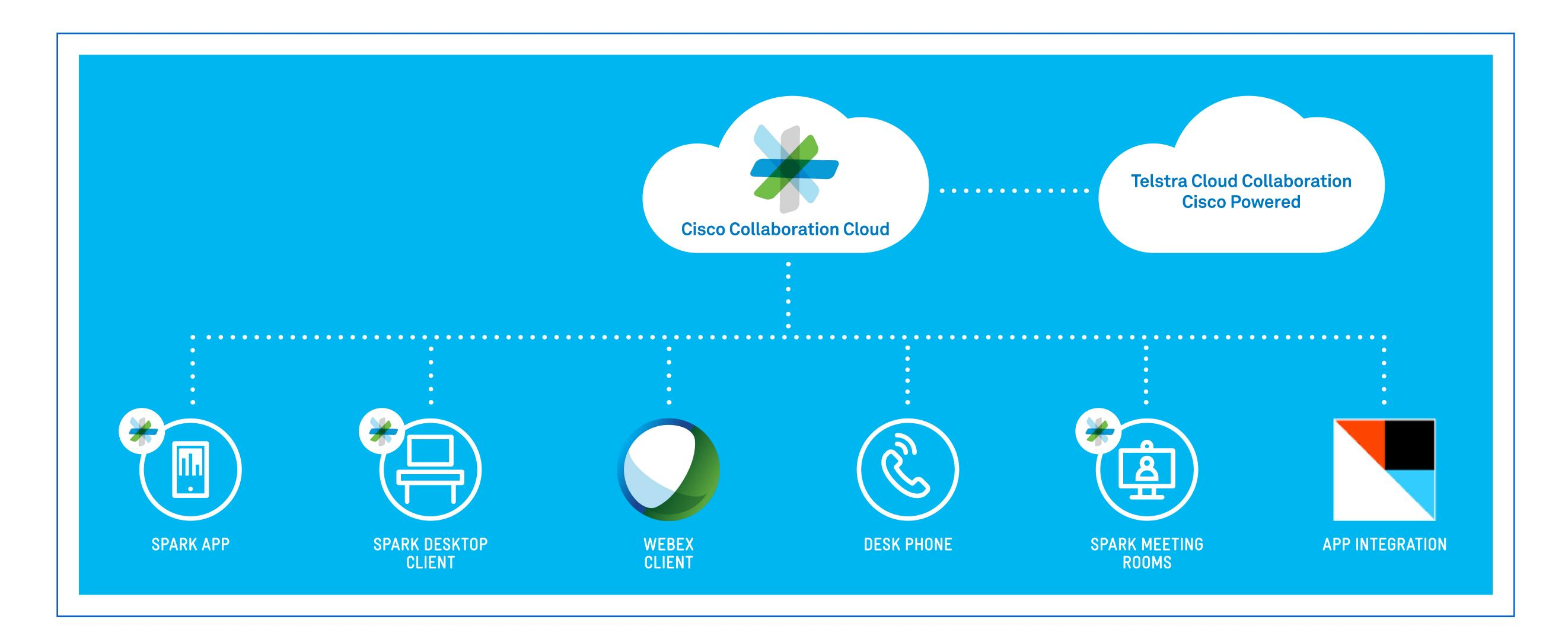
• Cisco® Collaboration Cloud Spark services are hosted securely in the Cisco cloud while media and key management servers and TCCCP are in the Telstra cloud. This provides high-quality audio and video while providing
