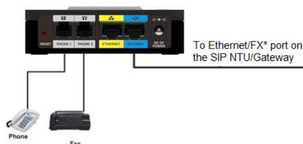
Figure 7: Cisco SPA122/ATA192 Rear connections
