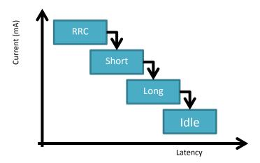
The point of all the above discussion is that it takes time, power and network signalling to switch between these RRC states and so it makes sense to minimize unnecessary state changes
