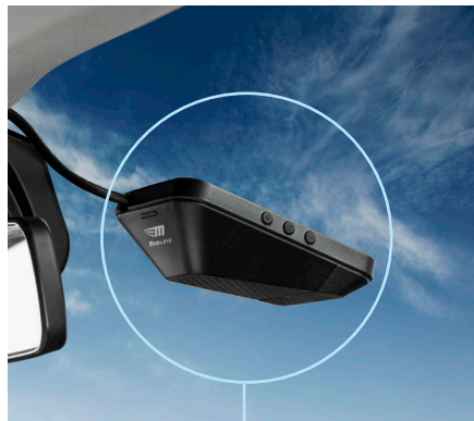
The camera unit containing the camera, EyeQ™ chip, and speaker, mounted on the inside of the windshield.
