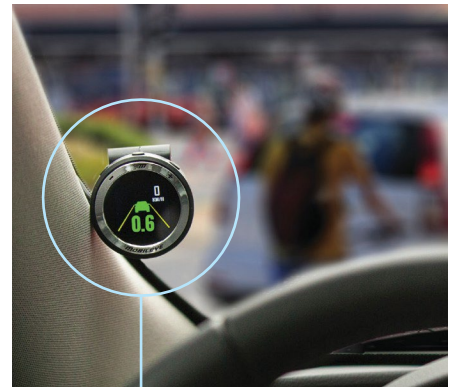
The EyeWatch™ display for visual alerts, mounted in vehicle's cabin.
